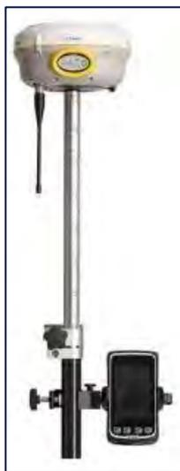
Figure 12: D-GNSS Trimble R8
